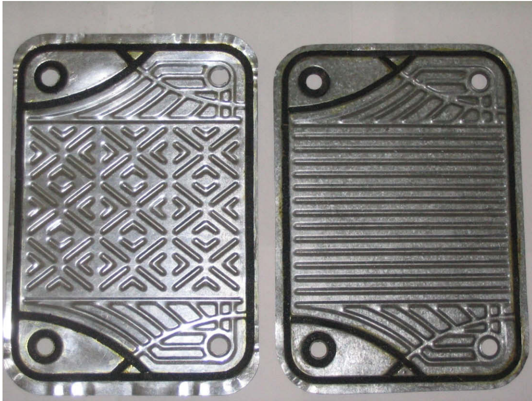
Fig. 2. The heat exchanger having the PHE corrugated and PHE asterisk surface structure.
